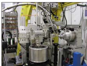
Sample Changer at 22-BM Beamline
