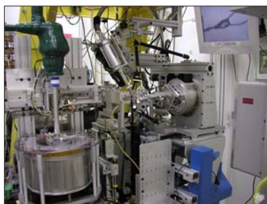
SER-CAT robot located at BM-22 endstation. Visible features from left to right: cryogenic sample changer, auto-mounter and computer display of crystal centering simplified by SERGUI. Mounting a crystal takes less than 5 seconds.
